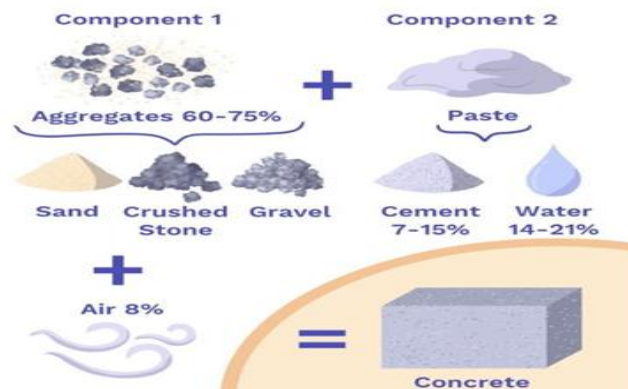
Fig 9. Composition of concrete
