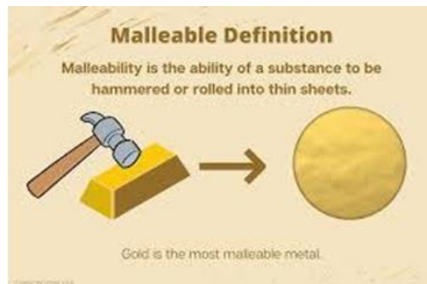
Fig 7 representation of malleability in a metal
